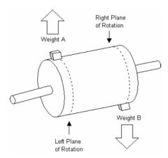
The couple unbalance can be compensated by two weights, which are positioned to counteract the couple unbalance at two planes. The ideal balancing task is to reduce the inhomogeneous mass distribution caused forces by adding or removing weights along the shaft.
